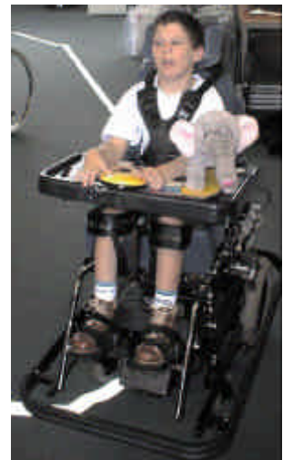
Pupil operating Smart Wheelchair using switch(es) instead of joystick.
