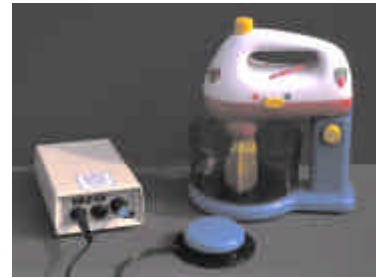
switch operation of a food mixer, through a control unit
