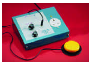
mains switcher unit
