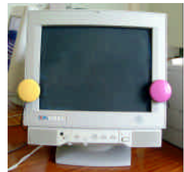
switches attached to the touch monitor
