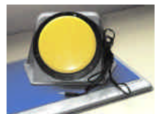
mounting a switch with a board and wedge
