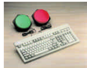
SwitchBoard with switches attached
