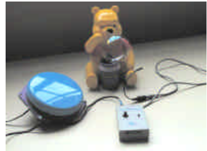
a toy control box that allows timer and latched modes - press the switch and teddy blows bubbles!
