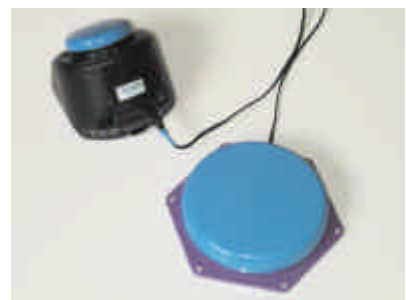
switch connected to a One Step communicator
